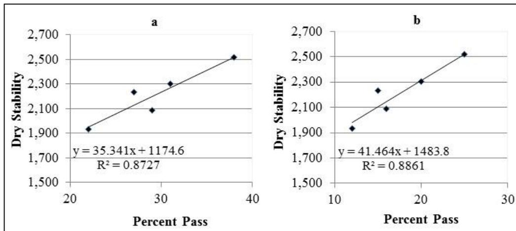
**Figure 3. Correlation between dry stability and percent passing a) sieve No. 8 and b) sieve No. 16**
