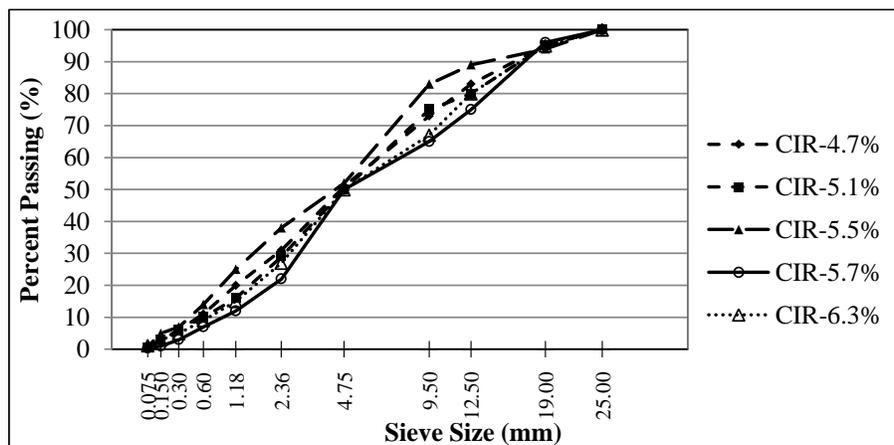
**Figure 1. Gradation of RAP samples**
