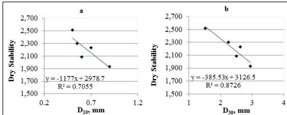
Figure 4. Correlation between dry stability a)  $D_{10}$  and b)  $D_{30}$
