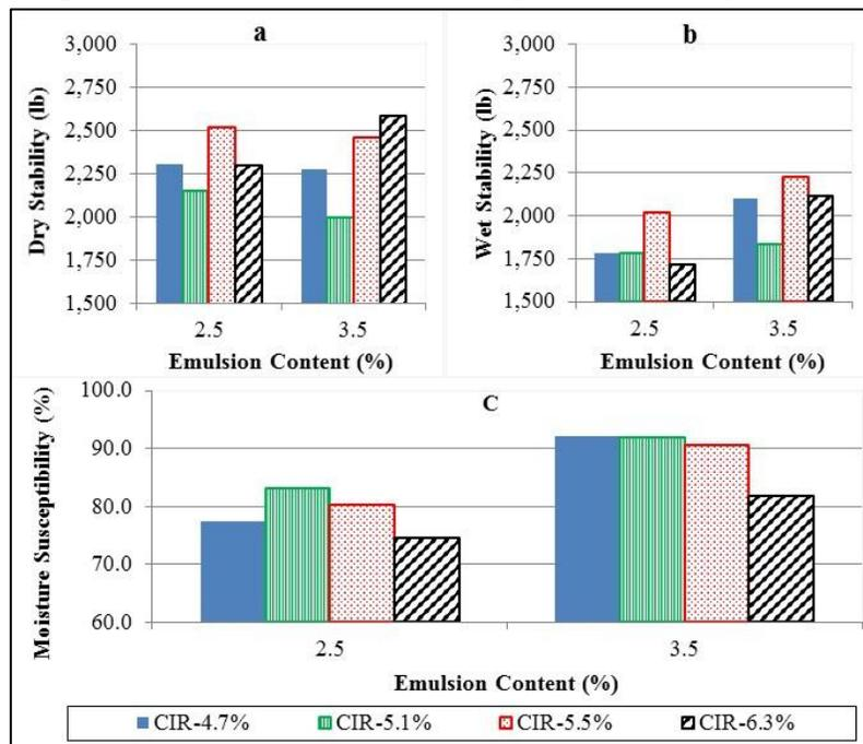
Figure 6. Effect of emulsion content on physical properties of cold-recycled mixes a) dry stability, b) wet stability, and c) moisture susceptibility
