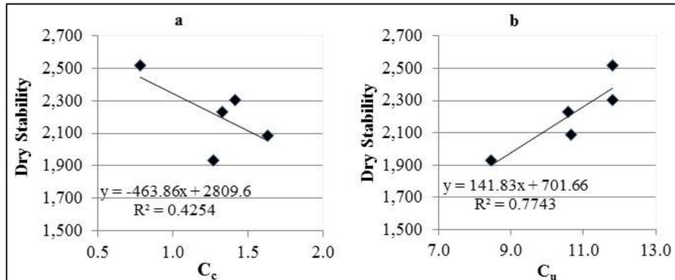
Figure 5. Correlation between dry stability a) coefficient of curvature and b) material uniformity coefficient
